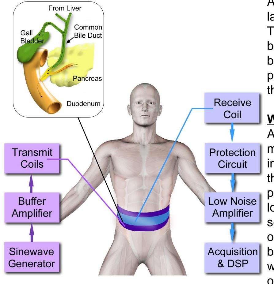
CollWireless Magnetoelastic Sensing:<br/>A resonant sensor, driven and<br/>measured by external coils, is<br/>integrated along the inner sidewall of<br/>the stent. The sludge accumulation<br/>process imparts viscous and mass<br/>loads on the sensor, altering the<br/>sensor resonant frequency. For<br/>optimal response, the sensor must<br/>be biased with a DC magnetic field,<br/>which can be provided with a layer<br/>on the stent.
