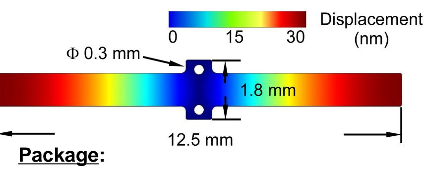
The sensor and the magnetic strips are packaged in a biocompatible flexible package to prevent damage during the surgery of implantation. Perforations in the package allow fluidic communication to the sensor. The package is then mounted on the inside wall of the stent.
