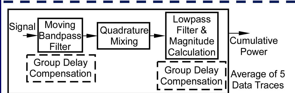
To increase the signal to noise ratio, several digital signal processing steps are implemented
