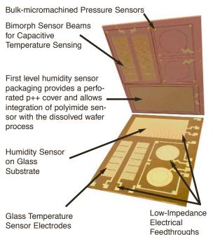
A MEMS chip measuring pressure, temperature, and relative humidity has been realized for an ultra-low-power environmental microsystem. The chip uses (1) a bimorph structure based on differential thermal expansion for sensing temperature and (2) a polymer structure based on moisture absorption for sensing relative humidity.
