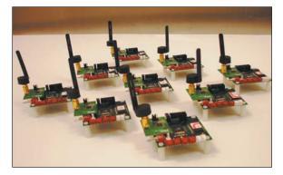
Figure 1 – Fully functional Narada wireless sensor network.
