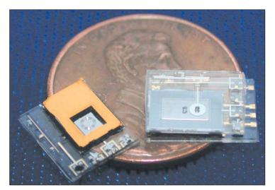
The bottom (left) and top (right) of the hybrid microvalve.
