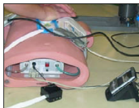
Figure 3 – The CPR Training Sensor is intended for use during actual CPR effort in the field. Sensory input and signal processing will result in more effective CPR delivery.
