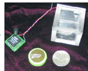
Figure 3 – The CPR Training Sensor is intended for use during actual CPR effort in the field. Sensory input and signal processing will result in more effective CPR delivery.
