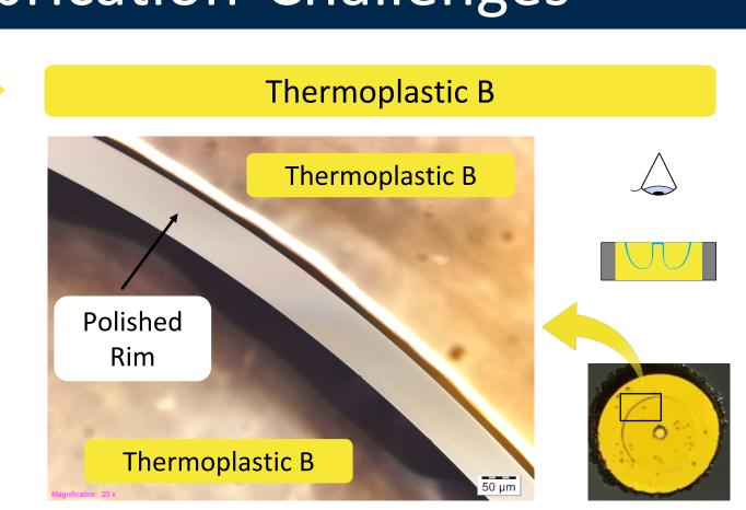
Thermoplastic holds the shell in place during polishing. A smooth rim helps achieve a high quality factor by reducing micro-cracks and thermoelastic dissipation. Switching from Thermoplastic A to B produces far better results.
