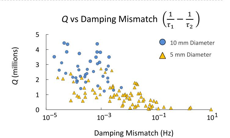
Resonant frequency is consistent. The addition of a protective coating before lapping and polishing improves quality factor repeatability. There is a strong correlation between damping mismatch and quality factor. This indicates the importance of symmetry, both in structure and surface condition.
