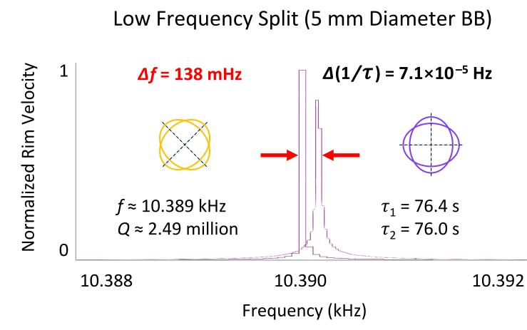
In 2013 our longest ring-down was 8 seconds. Fabrication improvements led to a >32× increase, paving the way to high-precision micro-gyros.
