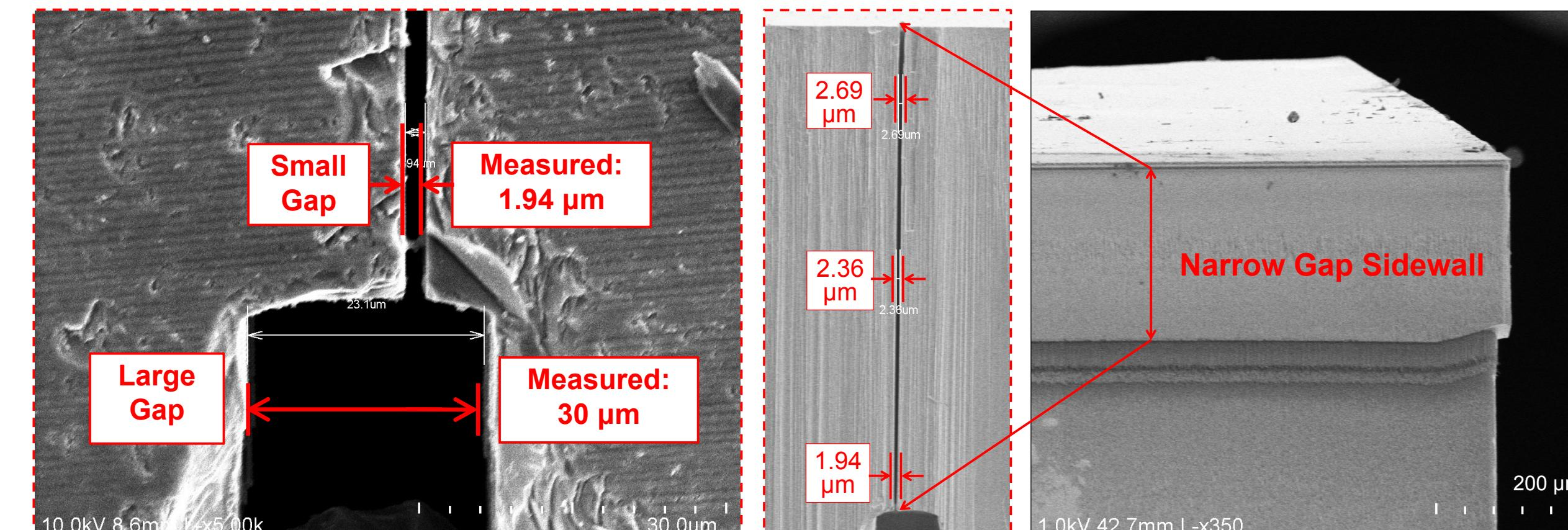
Two-gap CMOS Compatible Dry-Release Process
