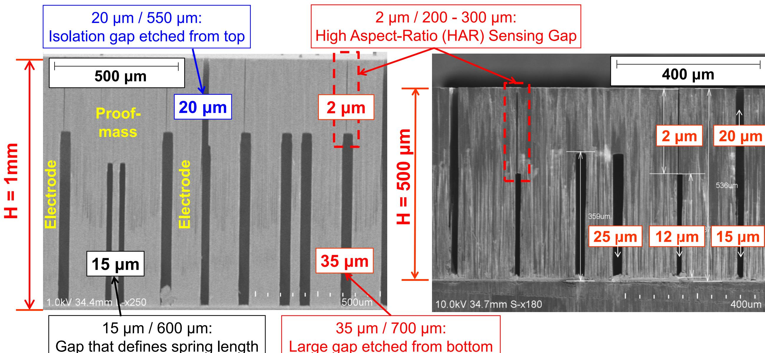
High aspect-ratio Narrow Gap  $2\mu\text{m} / \sim 250\mu\text{m}$
