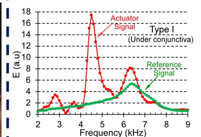
The Type I actuator was measured with the conjunctiva layer in place (Bottom).
