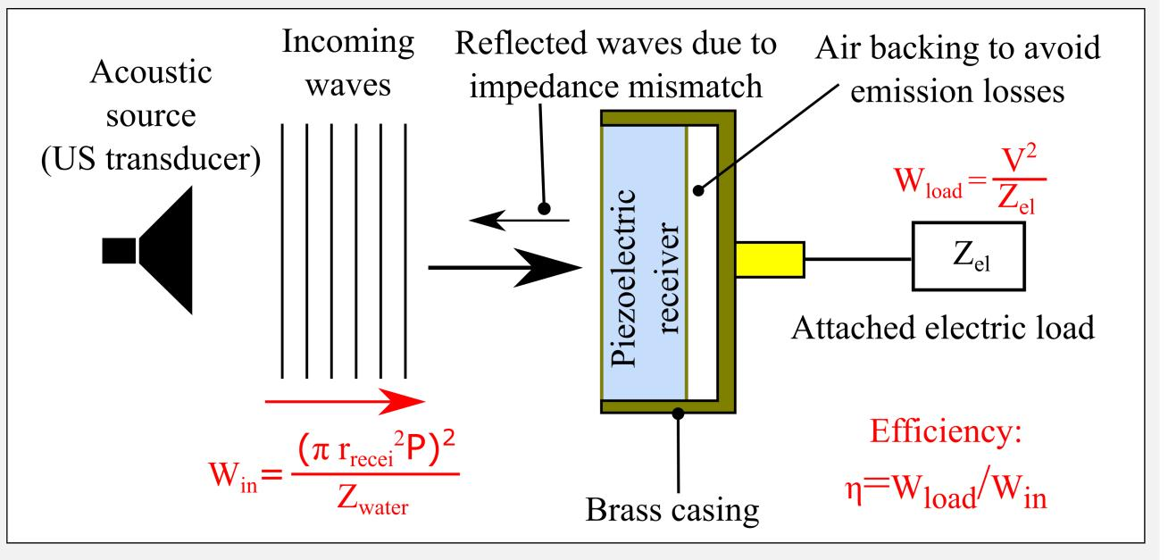
O Critical variables that influence the efficiency: • Acoustic attenuation  $(Q_m)$  & dielectric losses  $(\delta_{tn})$ • Front acoustic impedande mismatch (Reflection R)  $\circ$  Air at the back  $\rightarrow$  Perfect reflection and no losses
