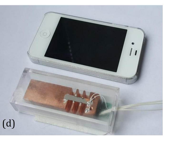
Fig. 1 (a) structure of accelerometer based on asymmetric-gapped cantilever; (b) structure of a conventional accelerometer; (c) decomposition of the bending of asymmetric-gapped cantilever; (d) an ultrasensitive accelerometer in comparison with an iPhone 4 smart phone.
