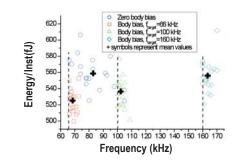
Different body bias configurations minimize energy and performance variability in 20 dies measured at Vdd=300mV.
